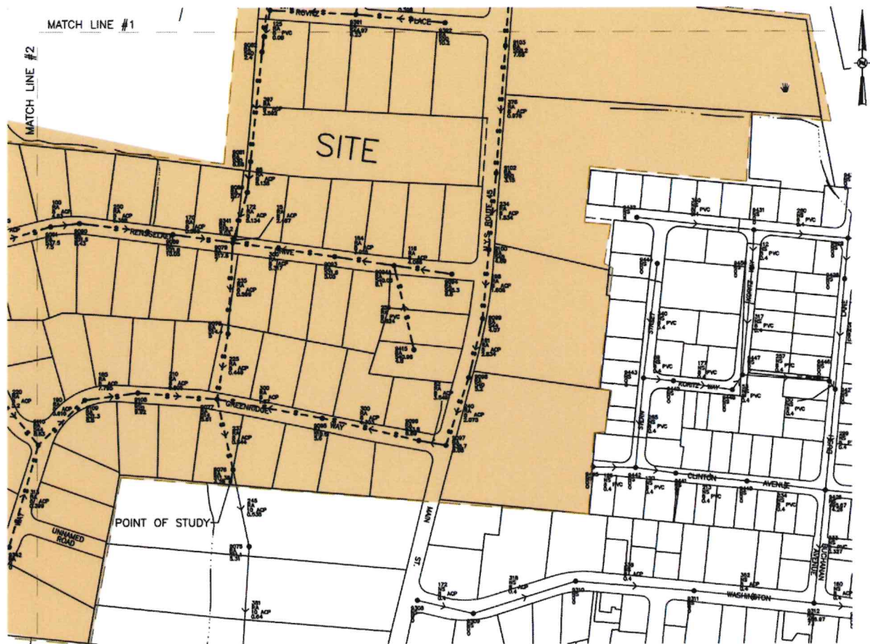
Partial plan of sanitary sewer services
