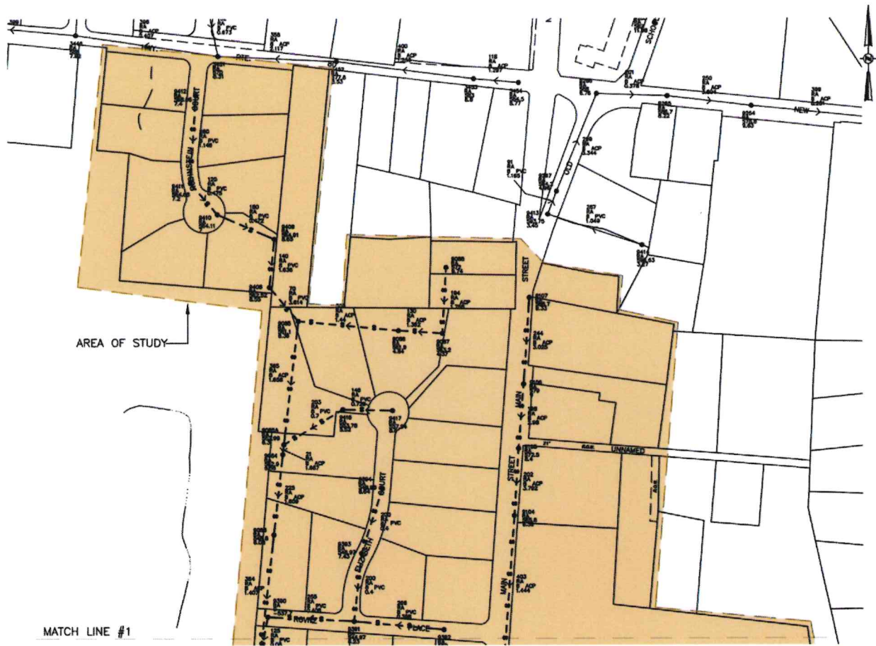
Partial plan of sanitary sewer services
