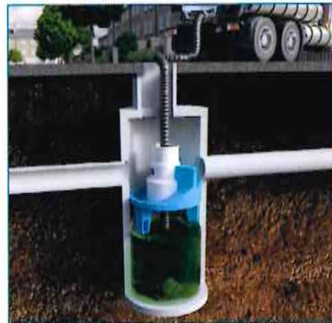
Fig 3. Maintenance is done with a vector truck
